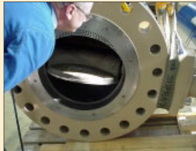
Fig. C: Special baffle ring used to increase the rangeability > 1:100
