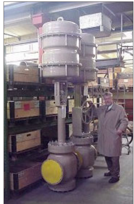
Fig. 39: Pneumatic diaphragm actuators, up to an effective diaphragm area of 5600 cm 2 , can offer a maximum initial spring force of 120 KN. Photo shows also the author of this paper.
