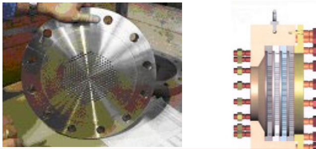
Fig. 12: Case study 2: Calculation and construction of downstream resistance structures like single and multi-baffles.
