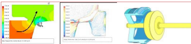
Fig. 13: Case study 2: CFD optimization of anti-cavitation trim design - computer flow simulation. Shown is SAMSON's AC Trim I System Parabolic plug top and seat guided. Seat and plug CFD optimized.
